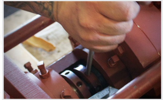
Tightening the main cylinder packing nut to snug.
