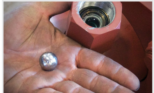
Remove ball and inspect all sides to ensure proper performance.
