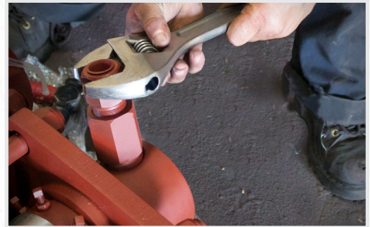
Removing the intake manifold.
