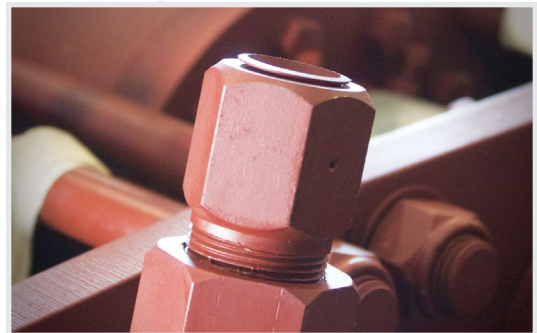
Weep holes located on the check cages.
