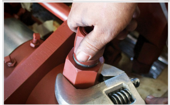
Careful remove manifold so the spring and ball stay in place.
