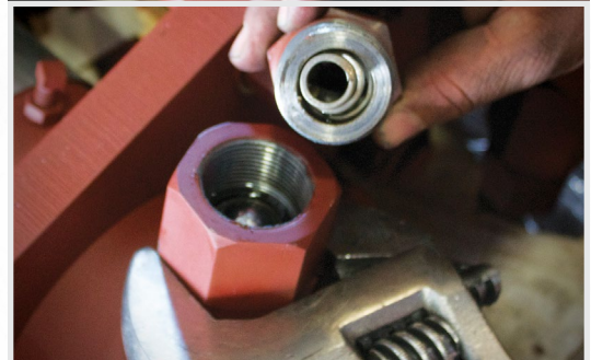
Inspecting the spring, ball and seat, and seal.
